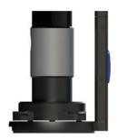
**6** Check that the button locks and that the collimate plate has no contact with the lower part of the Zfx<sup>™</sup> Synchronizer.
